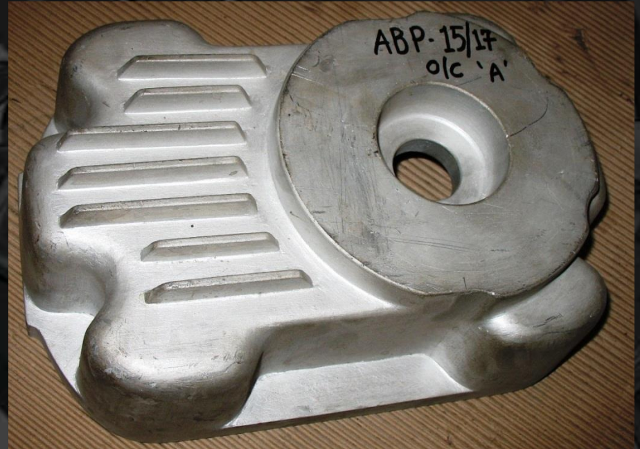
Aluminum Pattern for the component for C I Casting
